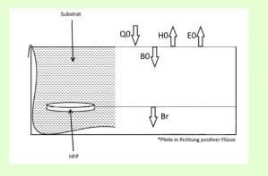
Figure 1 - **Energy balance on the green roof:** The main driving factor is the net radiation (Q0), which is partitioned into the latent heat flux (E0), sensible heat flux (H0) and soil heat flux (B0). The measurement of the soil heat flux in the substrate (Br) can be performed by heat flux plates (HFP) in the substrate only at a reference depth. In general,  $B0 \neq Br$ , as the layer between the two points stores energy.
