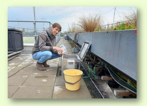
Figure 3: Johannes Stüllein calibrating roof runoff measurements. Author: Lucie Moeller (UBZ, UFZ)
